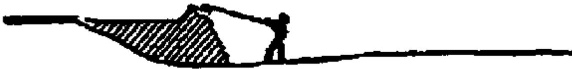
5. Every day the levelled wastes and the flanks are covered by between 15 cms and 25 cms of soil, sand, ash or composted wastes, etc. Daily or weekly the working face is covered to form an enclosed cell of wastes.
