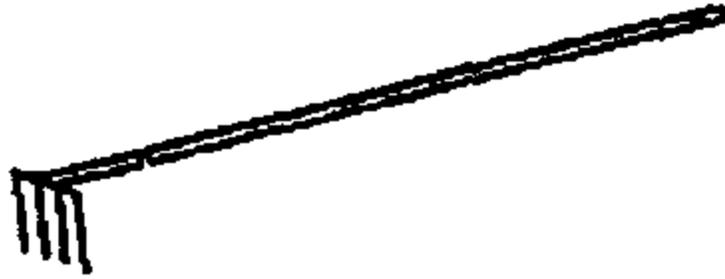
4. The heaps of wastes are levelled by a three-tine drag (or rake) with a handle about 2 metres long and the flanks are formed to an angle of about 45°. Levels and strip width are guided by pegs driven earlier.
